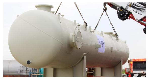
Also for both of items platforms and stairs are supplied. Gas boot is designed to separate production fluids into their constituent components of oil, gas, and water. Separator designates a pressure vessel for separating well fluids produced from oil and gas wells into gaseous and liquid components. They are normally used on a producing lease or platform near the wellhead, manifold, or tank battery to separate fluids produced from oil and gas wells into oil and gas or liquid and gas.
